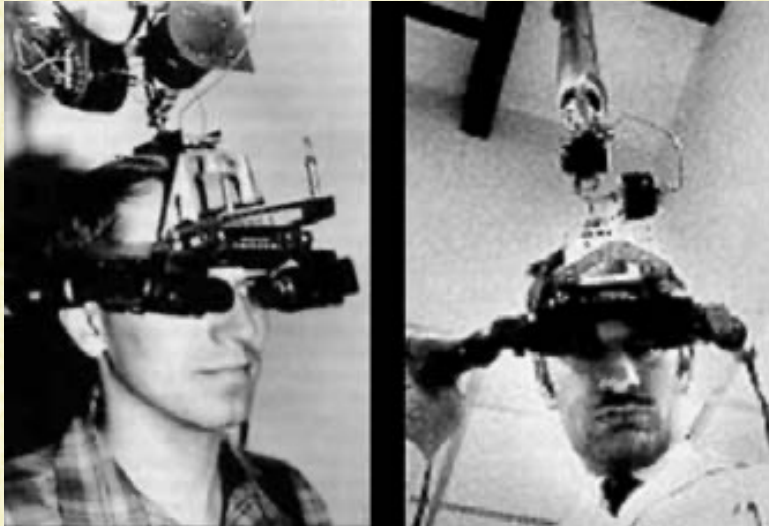
Ivan Sutherland: Head-mounted displays, with mechanical tracker
