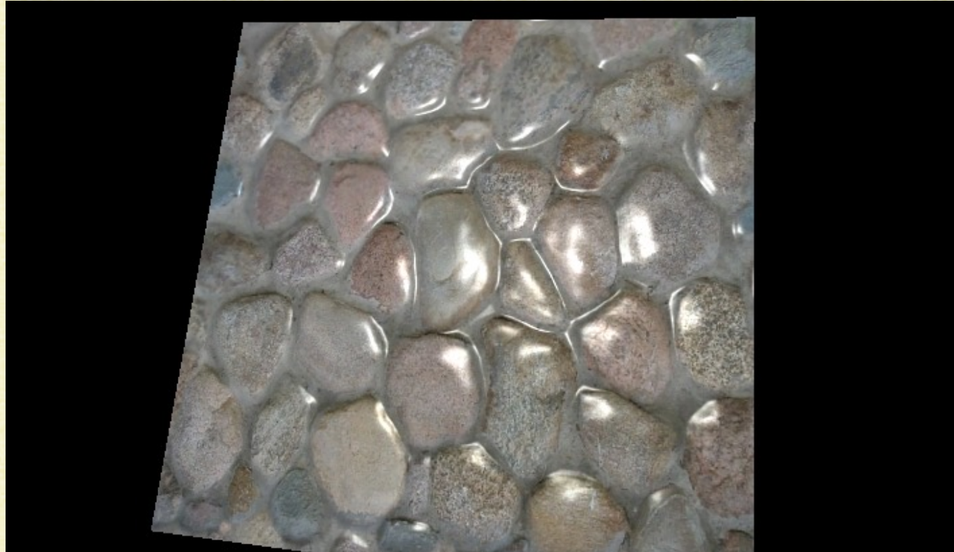
normal mapping on a plane (note the variation in specular highlights created by variation of the normal)
